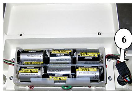
Figure 2: Display Cable Connector and Battery Compartment
