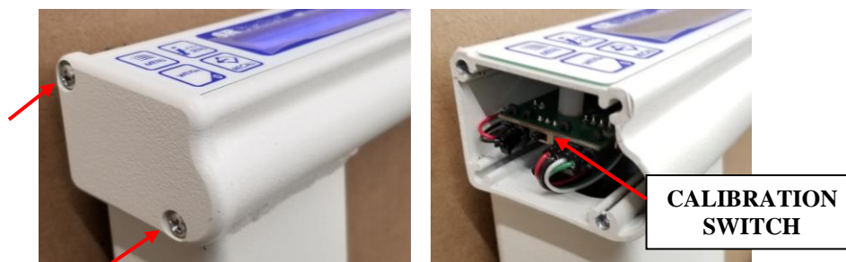
Figure 5: Calibration Switch Location
