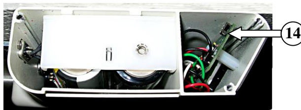
Figure 12: Display Board Calibration Switch Location
