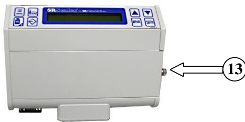
Figure 9: Battery Compartment Panel Screw
