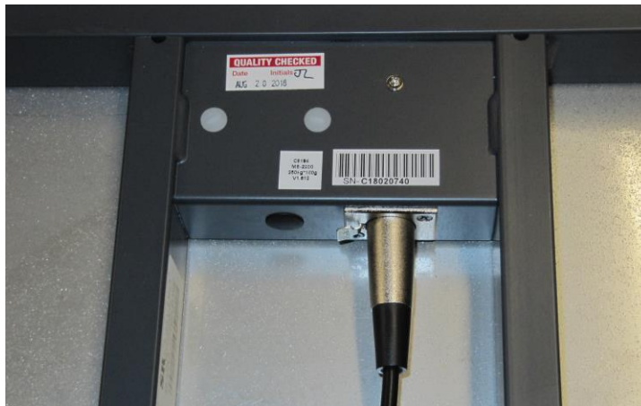
Figure 2: Cable Connection to Platform
